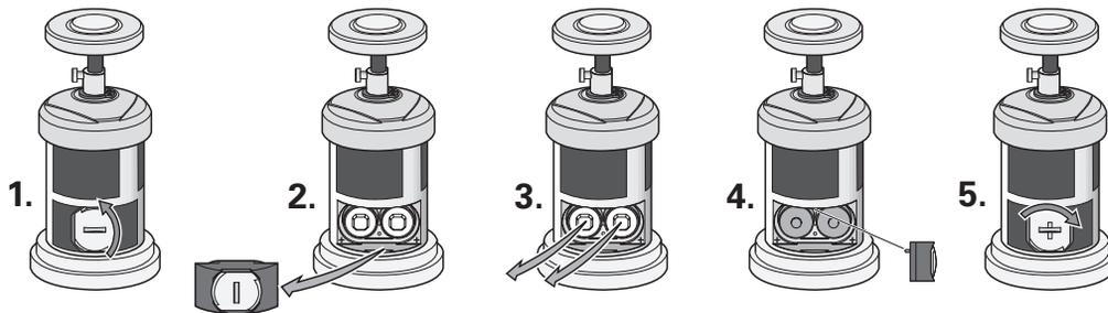
Remove the battery's protective cap before initial operation.
