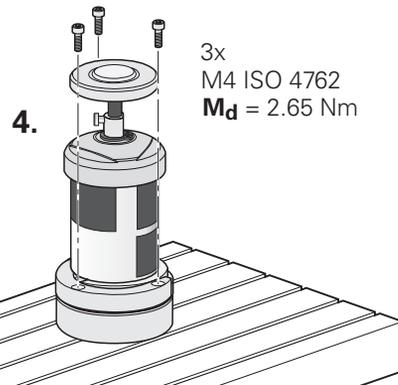
**Exchanging the connection pin / probe contact**
