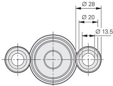
Mounting with fixing clamps
